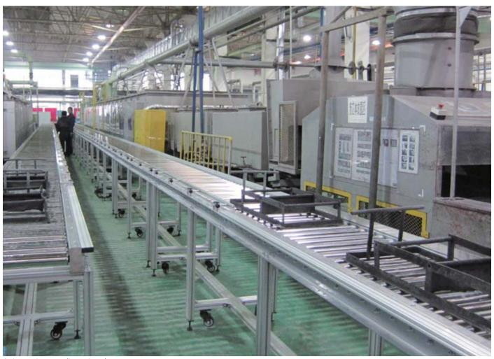
Carbon steel conveyor (for steel parts)
