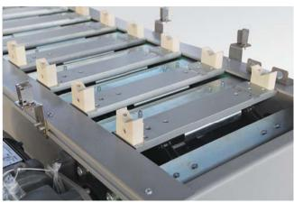
Chain conveyor with workpiece
