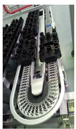
Conveyor with aluminum structure (for tooling pallet)
