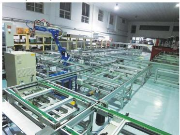
Automation assembly line (for rubber coating)
