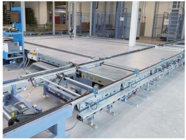
Heavy load capacity of chain conveyor (for 3000kg)
