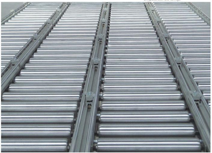
Zinc plated steel roller conveyor(automobile parts)
